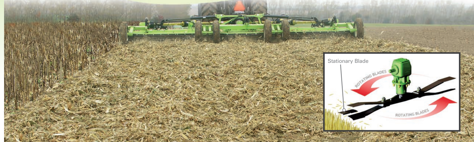
5026 fixed knife mulching corn
